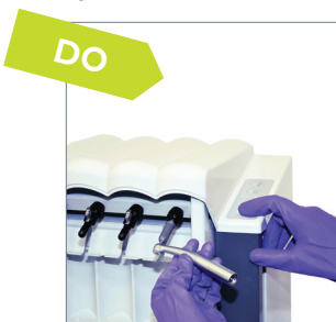
Weekly chuck care using the KAVO QUATTROcare Plus
