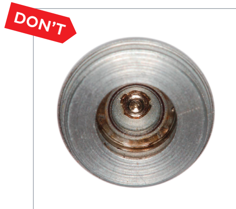
Push-button was abraded due to incorrect use
