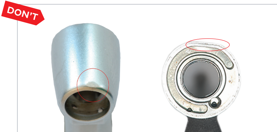
Handpiece showing damage from being dropped
